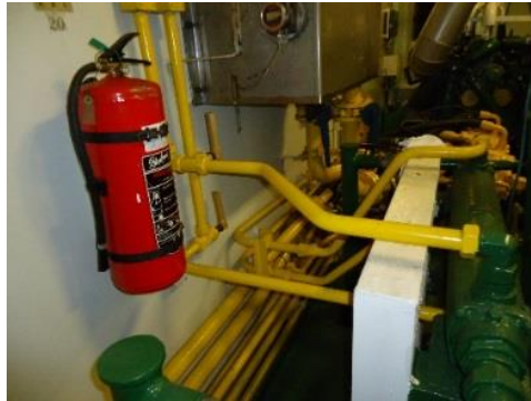
Detroit engine room (Schottel water jet engine) cooling systems for schottel and aircon systems.
