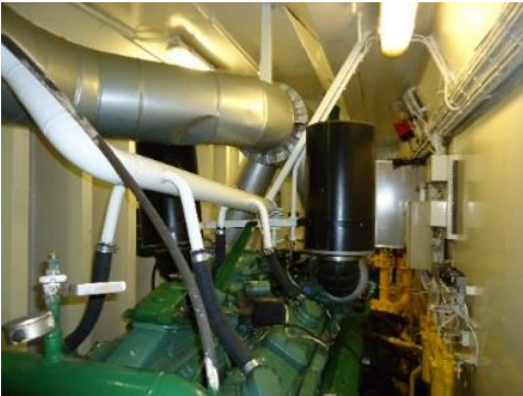
Detroit engine room (Schottel water jet engine) cooling systems for schottel and aircon systems.
