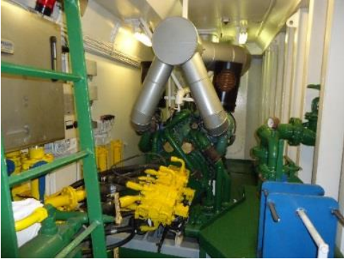
Detroit engine room (Schottel water jet engine) cooling systems for schottel and aircon systems.
