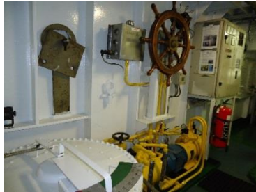
Steering gear room, deutz emergency generator
